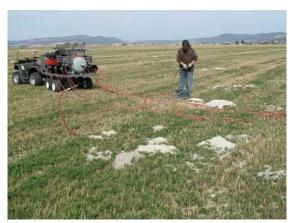
monoxide (CO) gas with the rodents reportedly killed before they escape the burrow. Kohler Co. engines are exclusively used to power the H&M Gopher Control equipment.
